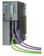
\*\*\*\*\*\*\*\*\*\*\* Replacement part \*\*\*\*\*\*\*\*\* SIMATIC S7-400, CPU 416-3 PN/DP Central processing unit with: work memory 16 MB, (8 MB code, 8 MB data), Interfaces: 1st interface MPI/DP 12 Mbit/s, (X1), 2nd interface Ethernet/PROFINET (X5), 3rd interface plug-in IFM module (IF1)
